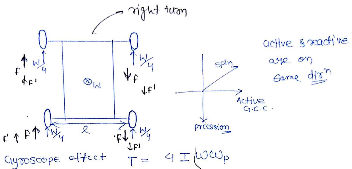
$$\text{Speed of vehicle} = \underline{V = \gamma w = R w_p}$$
