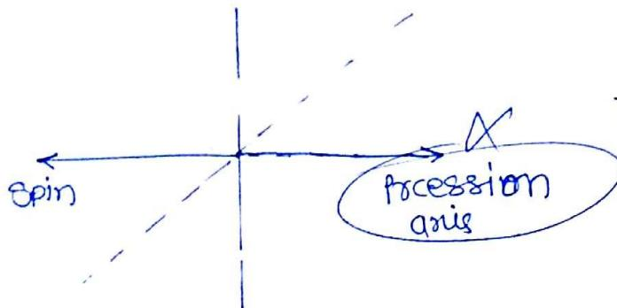
\* There is no reactive gyroscopic effect on ship during rolling
