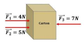
**Solution:**  $F_1 = 4$  N and  $F_2 = 5$  N are the forces acting on the carton box in the same direction.
