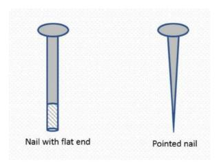
**Solution:** The pointed nail covers a smaller area on the wall than a flat end nail. As a result of which pressure exerted by the pointed nail on the wall is greater as compared to the pressure exerted by the flat end nail on the wall.
