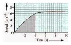
The part of the graph in red colour between time 6 s to 10 s represents uniform motion of the car.
