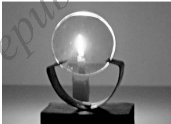
Fig. 15.27 Image formed by a concave lens
