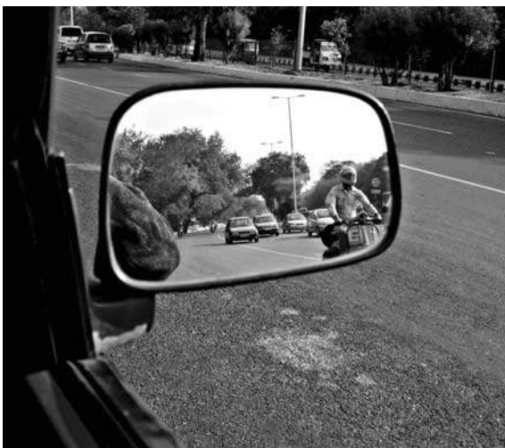
Fig. 15.20 Convex mirror as side view mirror
