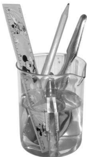
Fig. 4.8 Conduction of heat by different materials
