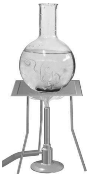
Fig. 4.9 Convection of heat in water
