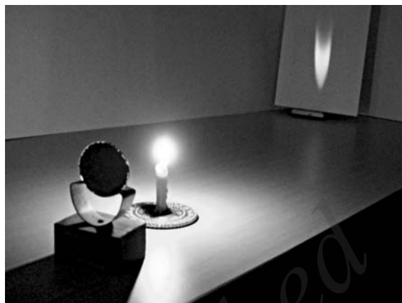
Fig. 15.15 Real images formed by a concave mirror
