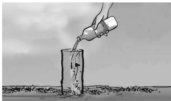
Fig. 9.5 Measuring rate of percolation
