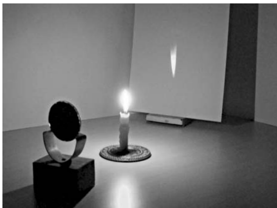
Fig. 15.15 Real images formed by a concave mirror
