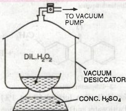
FIGURE 11.12. Vacuum Desiccator.
