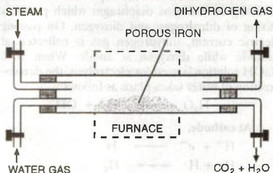
FIGURE 11.3. Manufacture of dihydrogen by Lane's process.
