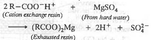
Thus, the water which comes out from the bottom of the first tank is richer in  $\text{H}^+$  ions. This water is then passed through a second tank which is packed with anion exchange resins supported
