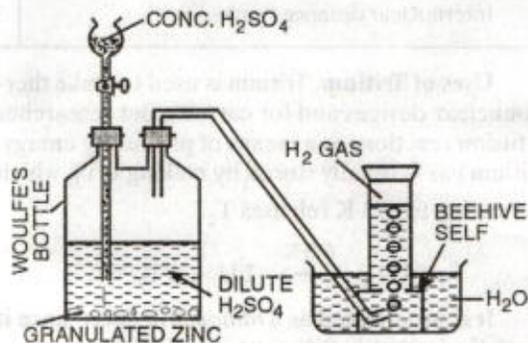
FIGURE 11.2. Preparation of dihydrogen gas in the laboratory.
