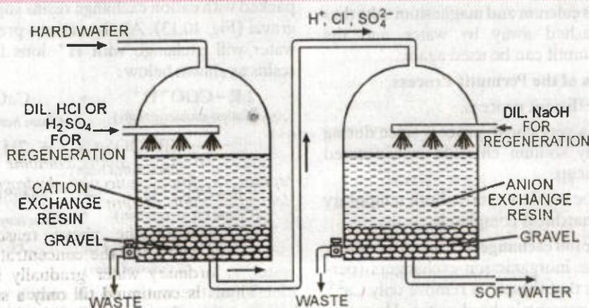
FIGURE 11.9. Ion exchange process involving organic resins.
