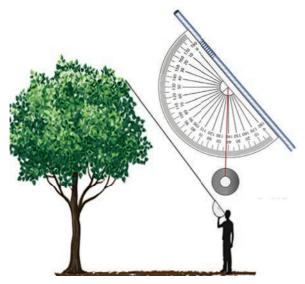
string should hang down freely, crossing the protractor portion of the clinometers. Read the angle shown, and subtract from 90° to find your angle of vision from your eye to the top of the tree (it can be helpful here to have an assistant to read the measurement while we look through the straw). We record our results on a paper. From the spot, the clinometers ( read by assistant) show 55°. Subtracting from 90° that indicated that we looked at an angle of 35° to the top of the tree.
