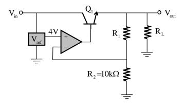
For a load R<sub>L</sub> drawing 200 mA, the maximum power dissipation in Q<sub>1</sub> (in Watts) is \_\_\_\_\_.
