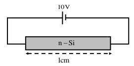
The donor doping concentration  $N_D$  and the mobility of electrons  $\mu_n \, are 10^{16} \, cm^{-3} \, and 1000 cm^2 V^{-1} s^{-1}$ , respectively the average time (in  $\mu s$ ) taken by the electrons to move from one end of the bar to other end is \_\_\_\_\_\_.
