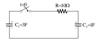
The switch is closed at time t = 0. The total energy dissipated (in Joules) in the resistor R until steady state is reached is \_\_\_\_\_\_.
