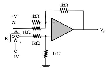
The value of  $\frac{V_{_{0B}}}{V_{_{0A}}}$  is \_\_\_\_\_\_.
