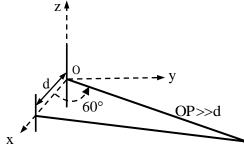
If the maximum radiated E-field at the point P in the x-y plane occurs at an azimuthal angle of  $60^{\circ}$  the distance d (in meters) between the antennas is \_\_\_\_\_.
