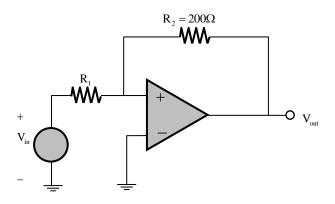
The value of  $R_1(\ln k\Omega)$  that gives a hysteresis width of 500 mV is \_\_\_\_\_.
