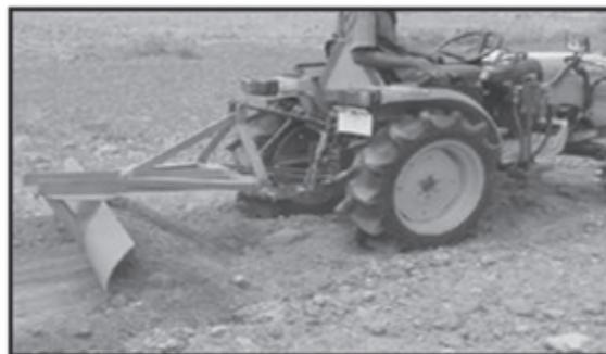
**Fig. 15.5:** Tractor drawn leveller
