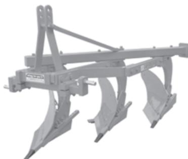
Fig. 15.1: Mouldboard plough
