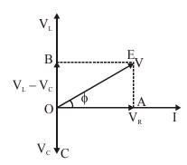
The effective opposition offered by L, C, R to a.c. supply is called impedance of LCR circuit and represented by Z.
