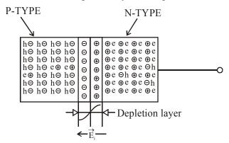
**Depletion layer:** It is the layer near the junction in which electrons are absent on n side and holes are absent on p side.
