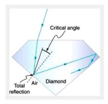
The total internal reflection of the light is used in polishing diamonds to create a sparking brilliance. By polishing the diamond with specific cuts, it is adjusted the most of the light rays approaching the surface are incident with an angle of incidence more than critical angle. Hence, they suffer multiple reflections and ultimately come out of diamond from the top. This gives the diamond a sparking brilliance.
