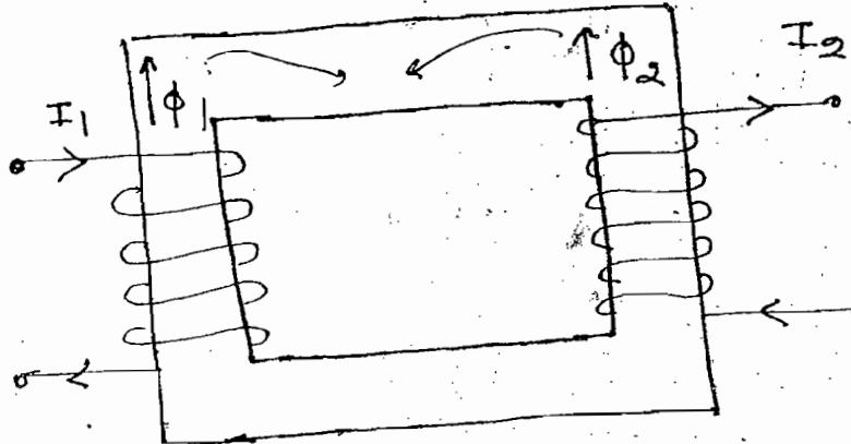
In above figure flux of the two inductors are completely closed path in opposite direction. Hence sign of mutually induced voltage is opposite to sign of self induced voltage.
