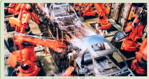
Figure 14.6: Robot welding the car body
