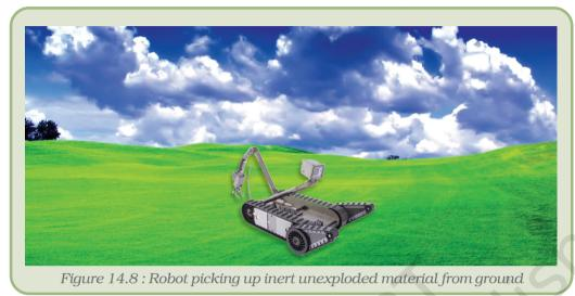
Security agencies also adopt such devices to locate explosives and unexploded material at public places like airports, industries railways, roadways and stations to name a few. These robots not only are able to detect the explosives beforehand but in some cases they can be also be used to de-circuit an explosive assembly without any human interface. This helps in reducing casualties of officers on duty in security agencies considerably.
