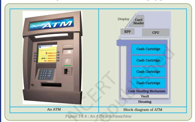
An ATM is a computer controlled machine designed to dispense cash, and other bank information without going to the bank. The ATM can also take deposits, transfer money between bank accounts along with basic banking services. This electronic machine is connected to the bank database through a computer controlled system that has capability to perform functions based upon the information that is provided by the customer through its banking card, it can be a debit card or credit card.
