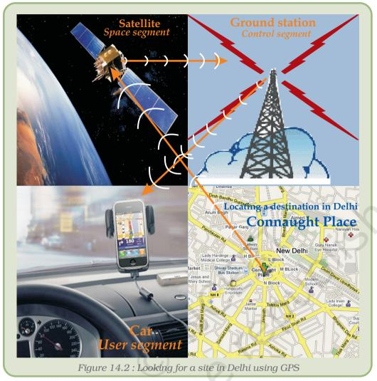
GPS has three segments. The **space segment** consists of 28
