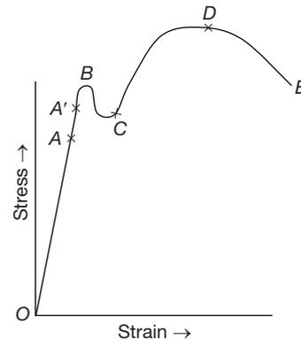
In the initial portion  $OA$ , stress is directly proportional to strain. Point  $A$  is the limit of proportionality. Slightly beyond  $A$ , when the load is released, strain disappears completely and original length is regained.
