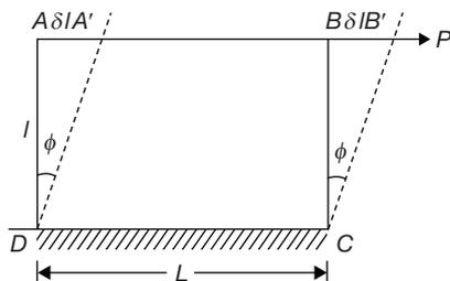
Shear strain  $\phi \cong \tan \phi = \frac{\delta l}{l}$
