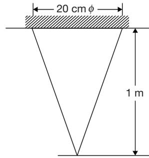
If specific weight is  $80000 \text{ N/m}^3$  and modulus of elasticity is,  $E = 2 \times 10^5 \text{ N/mm}^2$ , then extension of its length due to self weight is
