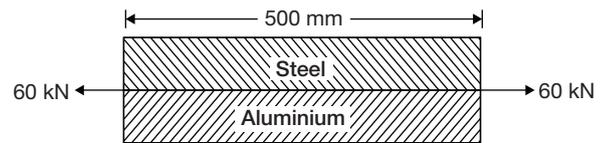
A compound bar of steel and aluminium of length 500 mm is subjected to an axial load of 60 kN. Area of cross-section of steel is  $750 \text{ mm}^2$  and aluminium is  $1000 \text{ mm}^2$ . Modulus of elasticity of steel and aluminium are  $2 \times 10^5 \text{ N/mm}^2$  and  $1 \times 10^5 \text{ N/mm}^2$  respectively. Load shared by steel and aluminium is in the ratio
