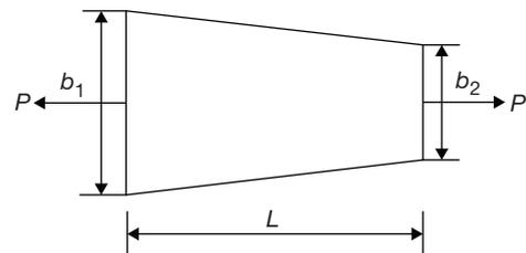
$$\delta L = \frac{PL}{tE(b_1 - b_2)} \log \frac{b_1}{b_2}$$
