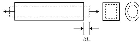
Within elastic limit, there is a constant ratio between lateral strain and longitudinal strain. This is known as Poisson's ratio.
