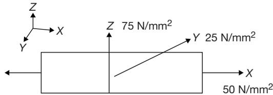
If Young's modulus of elasticity is  $150 \text{ kN/mm}^2$  and Poisson's ratio is 0.25, then what will be the strain in 'y;' direction?
