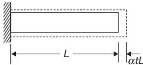
No stresses will be developed if the bar is free to expand. But, if the free expansion is prevented, then thermal stresses will be developed.
