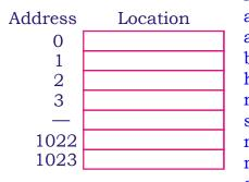
memory organization. Memory is organized as an array of bytes. A byte is basic storage and accessible unit in memory. Each byte is identifiable by a unique number called address. Suppose we have 1KB of memory, since 1KB=1024 bytes, the memory can be viewed as an array of locations of size 1024 with the subscript range (0 to 1023). 0 represents the address of first location; 1 represents the address of second location; and so on 1023 represents the address of last location.
