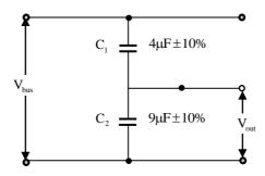
The measurement capacitors  $C_1$  and  $C_2$  have tolerances of  $\pm 10\%$  on their nominal capacitance values. If the bus voltage  $V_{bus}$  is 100 kV rms, the maximum rms output voltage  $V_{bus}$  (in kV), considering the capacitor tolerance, is\_\_\_\_
