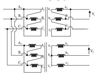
The phase difference (in degree) between voltage  $V_1$  and  $V_2$  is \_\_\_\_\_\_.
