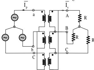
The line-to-line voltage rating is 230 V on the star side, and 115 V on the delta side. If the magnetizing current is neglected and  $\overline{I_s} = 100 \angle 0^{\circ} A$ , then what is the value of  $\overline{I_p}$  in Ampere?
