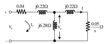
The "air-gap" voltage,  $V_g$  across the magnetizing inductance, is 210V rms, and the slip, is 0.05. The torque (in Nm) produced by the motor is \_\_\_\_\_.
