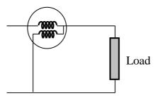
The wattmeter is connected as shown in the figure, to measure the power consumed by a load, which draws 25A at power factor 0.8. The voltage across the load terminals is 30V. The percentage error on the wattmeter reading is \_\_\_\_\_.
