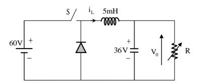
The output voltage V<sub>0</sub> is 36V. Assume that all the components are ideal, and that the output voltage is ripple-free. The value of R (in Ohm) that will make the inductor current (i<sub>L</sub>) just continuous is
