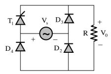
If the input voltage  $V_s$  is  $100 \sin(100\pi t)V$ , the average voltage across R (in Volt) under steady-state is \_\_\_\_\_.
