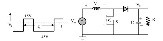
Also assume that the components are ideal, the inductor current is always positive and continuous and switching period is  $T_S$ . If the voltage  $V_L$  is as shown, the duty cycle of the switch S is \_\_\_\_\_\_.
