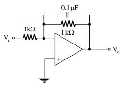
The amplitude of the output voltage V<sub>o</sub> (in Volt) is \_\_\_\_\_\_.
