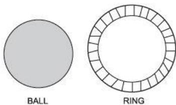
The metal ball can just pass through the hole of a metal ring formed out of a strip. When the ball is heated it gets stuck. But when the metal ring is heated,
