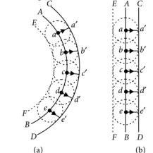
Huygens geometrical construction for the propagation of (a) spherical, (b) plane wavefront.
