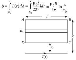
Induced emf set up into the loop
