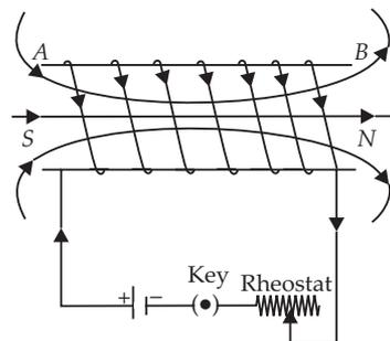
Figure shows the magnetic lines of force due to current carrying solenoid. The direction of current in the solenoid at the face A is clockwise, so it will have the south (S) polarity and the face B of the solenoid will have the north (N) polarity.
