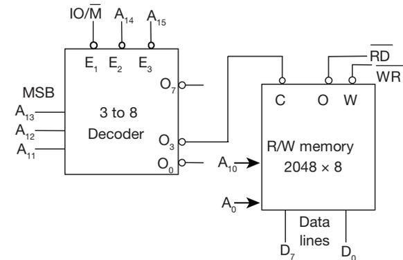
A R/W memory is interfaced with 8085 microprocessor as shown. What is the range of memory map connected to  $O_3$  line.
