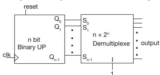
If the counter starts from reset, the above configuration works as
