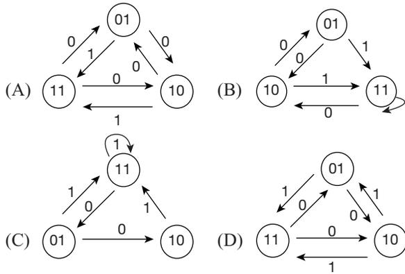
10. Find the state ( $AB$ ) diagram for the following sequential circuit?
