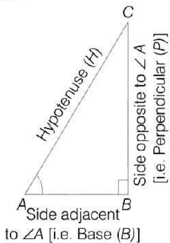
$$(i) \text{ sine } A \text{ or } \sin A = \frac{\text{Side opposite to } \angle A}{\text{Hypotenuse}} \left( \text{i.e. } \frac{P}{H} \right)$$
