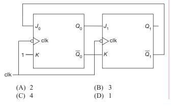
**18.** The counter shown above has initial state  $Q_2 Q_1 Q_0$ = 111(7), then the next states of  $(Q_2 Q_1 Q_0)$  (in decimal) are?
