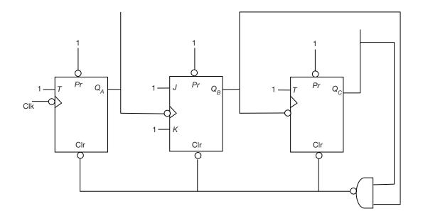
A counter formed with T, JK flip flops, as shown above, preset (Pr), clear (clr) are active low, asynchronous inputs, T, J, K are synchronous inputs. The modulus of the counter is:
