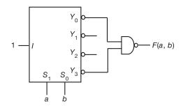
In the above circuit the function F(a, b) in POS form (A)  $(a+b)(a^1+b^1)$ (B)  $(a^1 + b)(a + b^1)$ (C)  $(a+b^1)(a^1+b^1)$ (D)  $(a+b)(a^1+b)$
