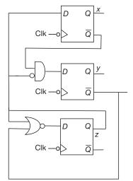
**32.** If at some instance prior to the occurrence of the clock edge x, y and z have a value 0, 1, and 1, what shall be the value of xyz after the clock edge?
