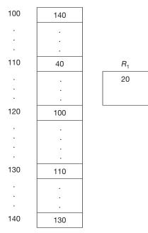
Assuming  $R_1$  is implied in the indexed addressing mode, what will be the actual value loaded into accumulator in immediate, direct, indirect and indexed mode respectively:
