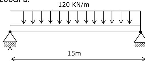
85. The beam is subjected to a maximum bending moment of
