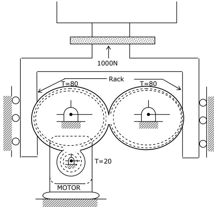
87. If the drive efficiency is 80%, the torque required on the input shaft to create 1000 N output thrust is
