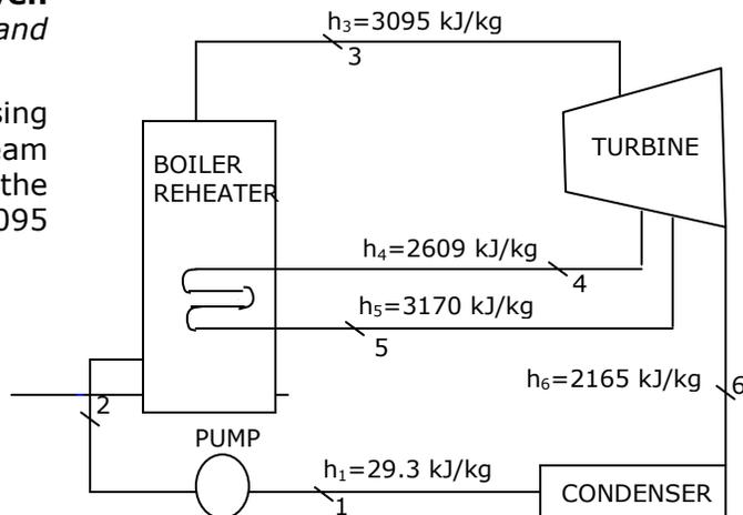
kJ/kg). After expansion in the turbine to 400 kPa ( $h_4 = 2609$  kJ/kg), the steam is reheated to 350°C ( $h_5 = 3170$  kJ/kg), and then expanded in a low pressure turbine to 10 kPa ( $h_6 = 2165$  kJ/kg). The specific volume of liquid handled by the pump can be assumed to be
