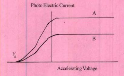
In the fig. shown, two monochromatic radiations of intensities  $l_1$  and  $l_2$  a  $(l_1 > l_2)$  having the same frequency are in turn incident on a photo sensitive surface causing photo electric emission. Curve A and B show the variation of photo electric current with accelerating potential. Identify the curves representing radiation with intensity  $l_1$  and  $l_2$  giving reason. Also give reason why the two curves have the same stopping potential  $V_0$ .
