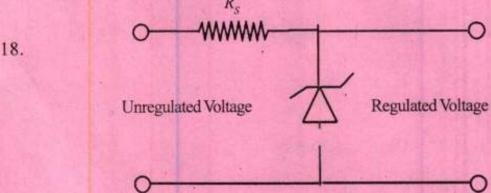
A zener diode of rating 100 mW is to be used as a voltage regulator. If the zener diode has the breakdown voltage of 5V and it has to regulate voltage which fluctuate between 3V and 7V, what should be the value of  $R_s$  for safe operation.
