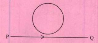
The electric current flowing in a wire from P to Q is decreasing. Find out the direction of the induced current in the metallic loop kept above the wire as shown in the figure.
