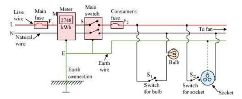
• Switches: It is a device which is connected in the live wire so as to turn 'ON' or 'OFF' the current in the circuit.
