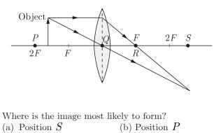
**60.** Rakhi conducts an experiment to produce an image of an object on a screen which is placed at 20 cm from the lens
