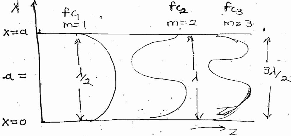
At exact cut-off frequency where  $\tilde{\gamma} = 0$ , the wave resonates b/w guide walls and oscillates b/w the walls for 'm' such frequencies.
