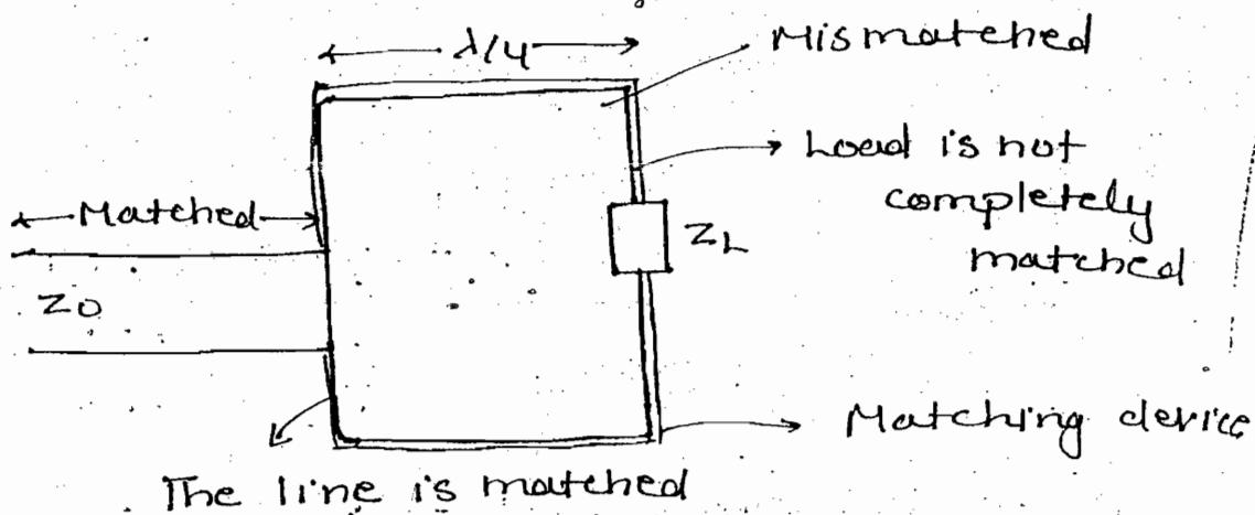
The termination of  $Z_0$  line is  $Z_{in}$  of  $\lambda/4$  matching device
