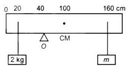
Rod will be in equilibrium, when net torque about point O will be zero. Torque at point O due to 2 kg mass
