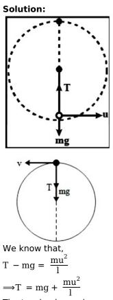
The tension is maximum at the lowest position of mass, so the chance of breaking is maximum.
