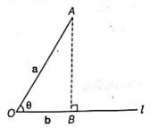
The ,the projection of OA on the line l is OB, which is given by  $|OA|\cos\theta$  and the direction of  $\vec{b}$ , called projection vector, being the same (or opposite) to that of the line l, depending upon whether  $\cos\theta$  is positive or negative.
