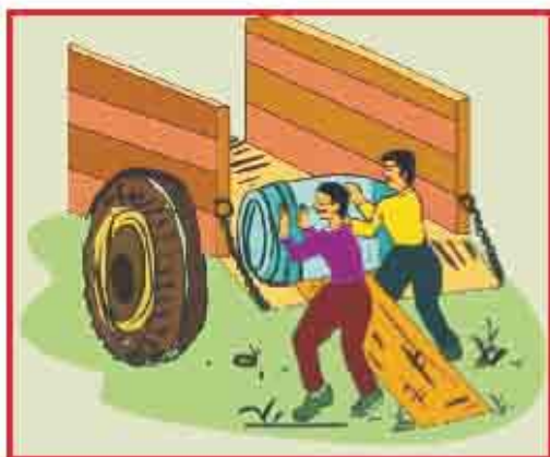
Figure 11.1 (a): To load a drum by an inclined plane Figure 11.1 (b): winding road up a hill
