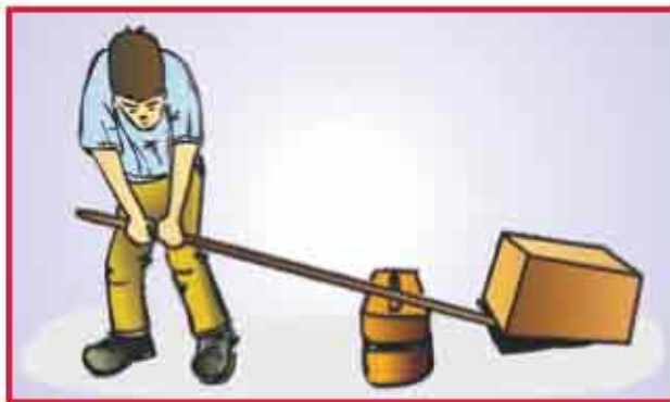
Figure 11.4 (b): Lifting a load with a bamboo staff
