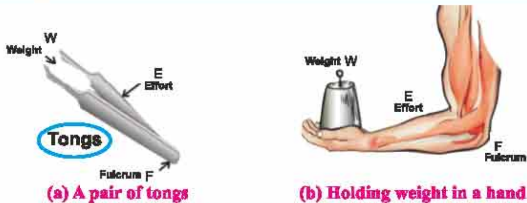
Figure 11.8 Examples of third order levers
