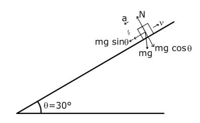
$ma = f_r + mg \sin\theta$   $ma = \mu mg \cos\theta + mg \sin\theta$   $a = (\mu \cos\theta + \sin\theta)g = (0.1\cos 30^\circ + \sin 30^\circ)10$  $= \frac{\sqrt{3}}{2} + 5 = 5.87 \text{ m/s}^2$
