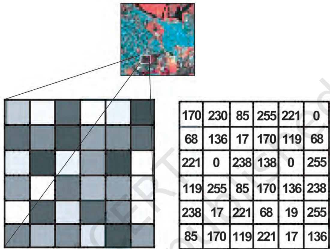
Figure 6.12 Digital Image (top) and Part of it zoomed showing Pixel's brightness (left) and the associated Digital Numbers (right)
