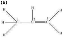
$C_1$  is  $sp^3$  hybridized, while  $C_2$  and  $C_3$  are  $sp^2$  hybridized.
