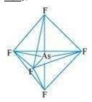
The central atom has no lone pair and there are five bond pairs. Hence,  $AsF_5$  is of the type  $AB_5$ . Therefore, the shape is\_trigonal bipyramidal.
