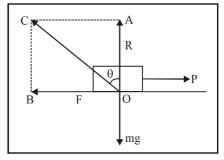
The value of angle of friction depends on the nature of materials of the surfaces in contact and the nature of the surfaces.
