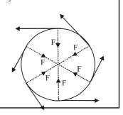
According to Newton's first law of motion, a body cannot change its direction of motion by itself. An external force is required for this purpose. It is this external force which is called the centripetal force.
