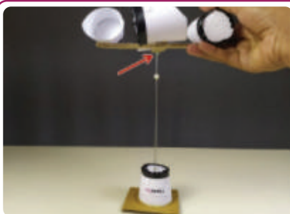
Fig. 7.9, The anemometer is assembled by inserting the cycle spoke through the straw fixed at the centre of the arms.
