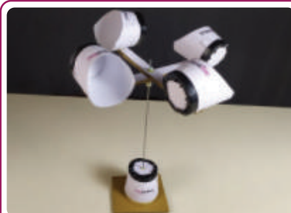
Fig. 7.10, The anemometer model is ready to record wind speed.
