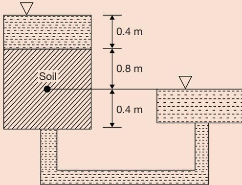
1. The total head, elevation head and pressure head in meters of water at the point  $R$  shown in the figure are
