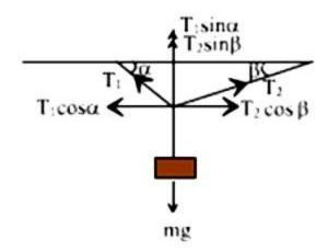
Considering components of tensions  $T_1$  and  $T_2$  along the horizontal and vertical
