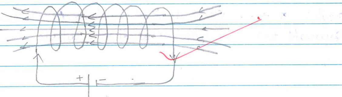
The magnetic field lines are ~~are~~ nearly straight and parallel to each other indicating that there is a uniform magnetic field inside solenoid.
