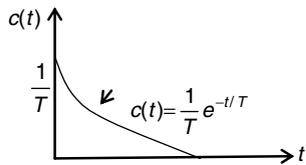
Figure 2 Unit-impulse response of first-order system.
