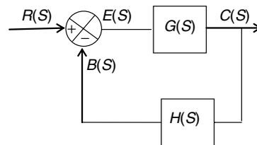
Figure 5 Feedback control system.
