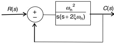
**Figure 3** Block diagram of standard second-order system.
