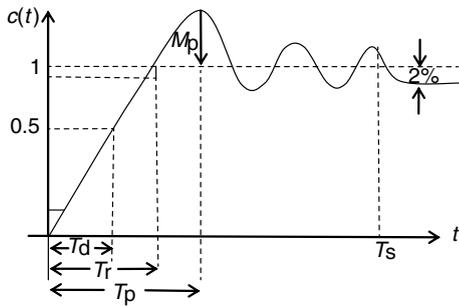
**Figure 4** Unit-step response of the under damped second-order system.
