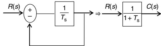
Transfer function of the system =  $\frac{C(s)}{R(s)} = \frac{1}{1+T_s}$
