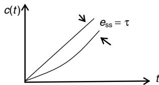
Figure 1 Unit-ramp response of first-order system.
