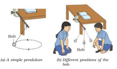
Fig. 7.10.1 Oscillation of a simple pendulum
