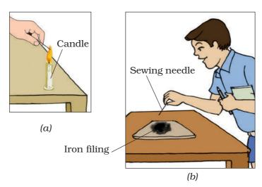
Fig.6.11.10 (ii) Magnet loses its strength on heating
