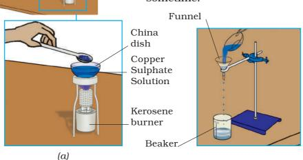
Fig.7.4.6 Arrangement to show the crystalisation
