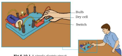
Fig.6.10.1 A simple electric circuit
