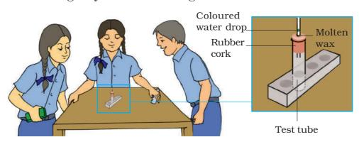
Fig.7.5.1 Arrangement to show expansion of air
