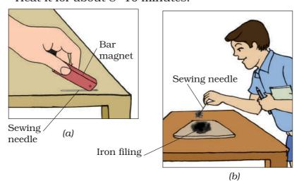
${f Fig.6.11.10}$  (i) Rubbing magnet over sewing needle
