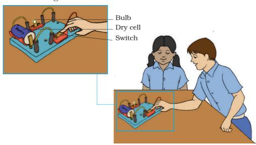
**Fig. 6.10.2** Circuit board connected with a bulb, switch and a cell
