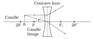
**Fig7.12.3** (a) Nature of the image formed bye using a concave lens
