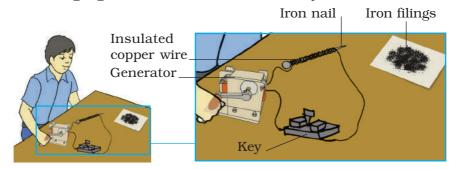
Fig.7.11.3 An electromagnet
