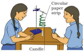
**Fig.7.2.6** Arrangement to show heat transfer in gases
