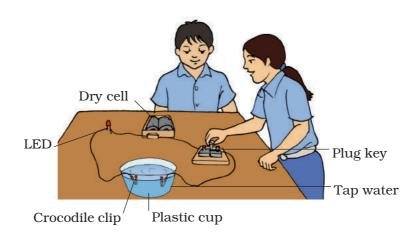
**Fig 6.10.4** Circuit arrangement using LED to test whether tap water conduct electricity or not
