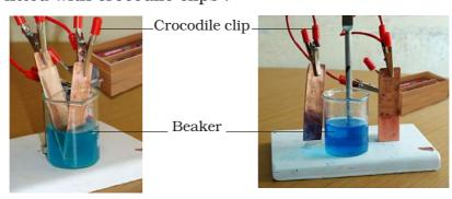
Fig.8.11.2 A simple electric circuit showing electroplating
