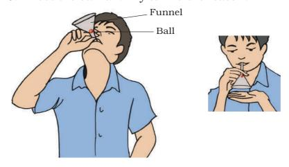
Fig.7.5.3 Arrangement to show air pressure
