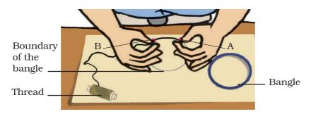
**Fig.6.8.2** *Measurement of the perimeter of the bangle*
