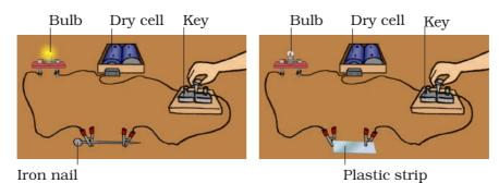
Fig.8.4.2 Testing good conductors and poor conductors
