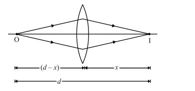
$$\frac{1}{f} = \frac{1}{v} - \frac{1}{u}, \qquad \qquad \frac{1}{f} = \frac{1}{x} + \frac{1}{d-x} = \frac{d}{x(d-x)}$$
