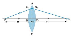
When a ray refracts from a lens (double convex), in above figure, then its image formation can be seen in term of two steps :
