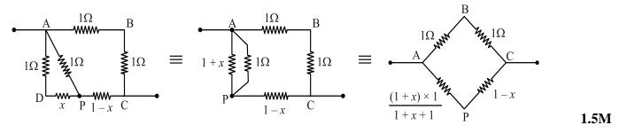
As the points B and P are at the same potential,  $\frac{1}{1} = \frac{\frac{(1+x)}{(2+x)}}{(1-x)} \Rightarrow x = (\sqrt{2} - 1) ohm$  **1.5**M
