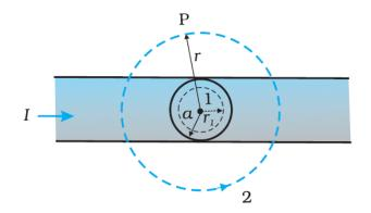
(a) Consider the case r > a. The Amperian loop, labelled 2, is a circle concentric with the cross-section. For this loop,  $L = 2 \pi r$
