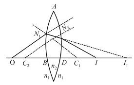
**Step 2:** The image of object O for first surface acts like a virtual object for the second surface. Now for the first surface ABC, ray will move from rarer to denser medium, then
