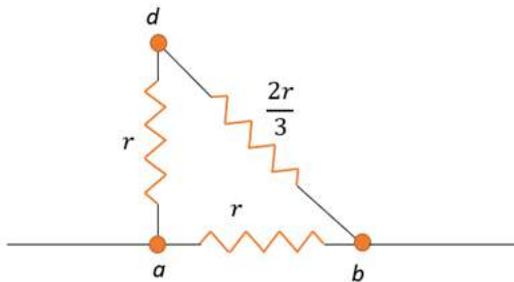
The resistor across  $db$  and  $ad$  are in series.
