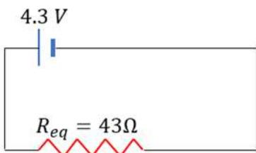
Now, the current that passes through  $R_{eq}$  also passes through the three series components : internal resistor,  $r'$  and ammeter.
