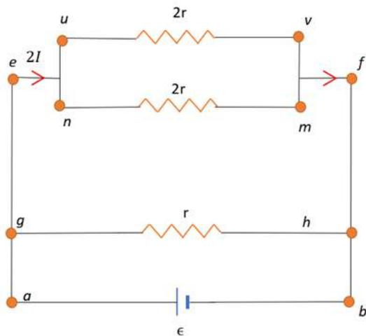
Clearly,  $uv$  and  $nm$  and  $gh$  are in parallel.
