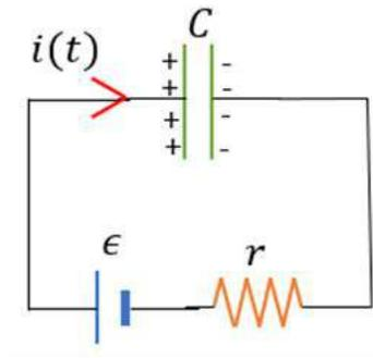
Let the potential across the capacitor  $C$  be at time  $t$  be  $V_c$ . Let the charge at time  $t$  be  $q$ .
