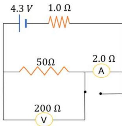
We will treat the measuring devices as ordinary resistors. Now, voltmeter and  $R = 50\Omega$  are in parallel. The equivalent resistance is given by:
