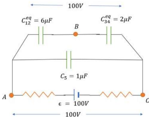
Now, the two capacitors  $C_{12}^{eq}$  and  $C_{34}^{eq}$  are in series.
