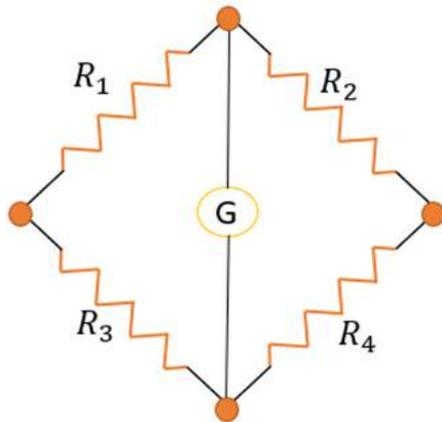
The condition for no deflection through the galvanometer is
