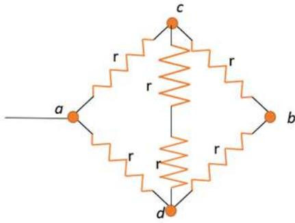
Note that there is symmetry in the circuit; the upper and the lower parts are identical. Hence, the potential at d should be the same as potential at c. Consequently, there is no potential difference across dc. We can neglect the resistors across dc.
