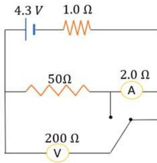
We will treat the ammeter and the voltmeter as ordinary resistors to find the equivalent resistance.
