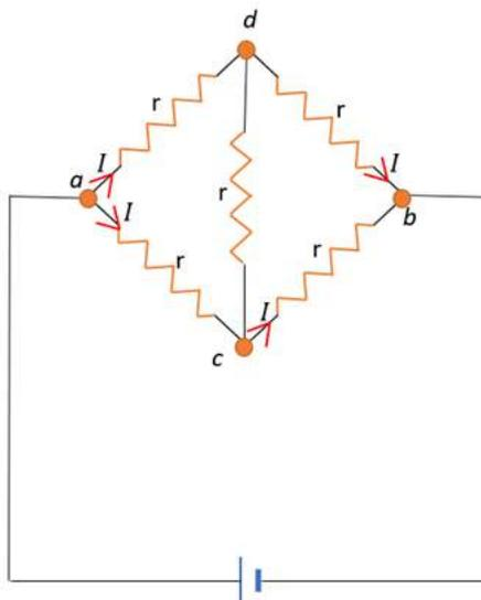
As we wish to find the resistance between points a and b, we have proceeded to add a voltage source of emf  $\epsilon$  between the points a and b.
