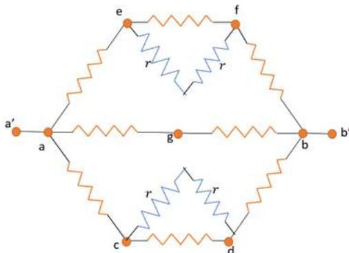
The blue resistors are in series. Net resistance =  $r + r = 2r$
