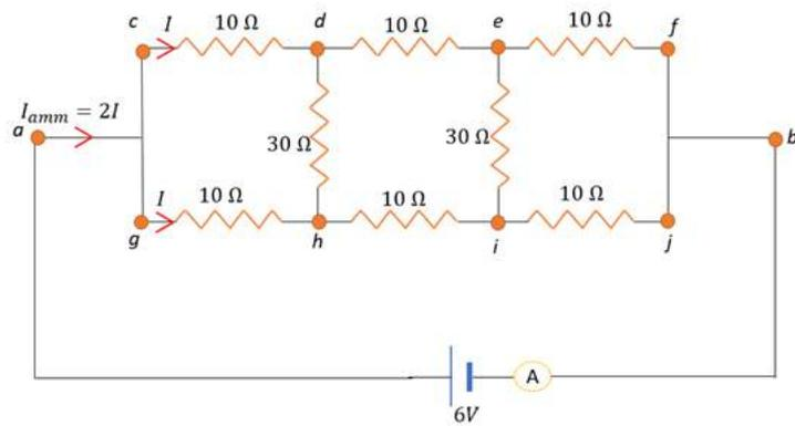
Due to this symmetry,  $d$  and  $h$ ;  $e$  and  $i$  are the same potential. Hence, no current passes through  $de$  and  $ei$ .
