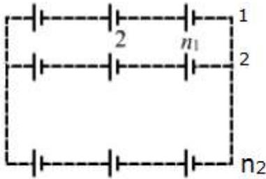
When  $n_1$  cells each with emf 'E' are connected in series, the total emf,  $E_{net}$  in one branch is,
