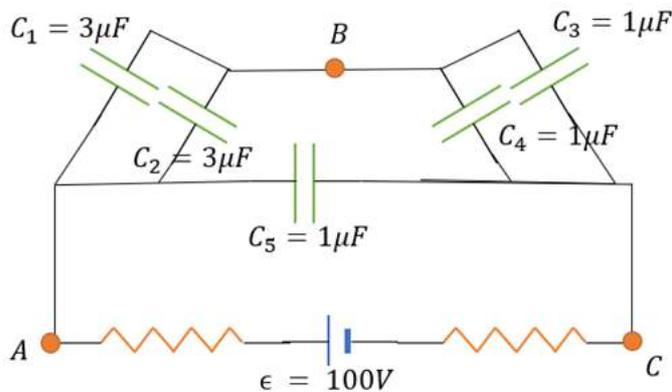
We can see that  $C_1$  and  $C_2$  are in parallel,
