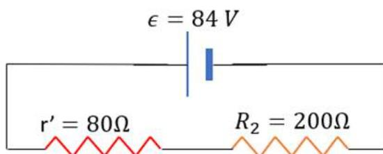
Note that  $r'$  and  $R_2$  are in series. The equivalent resistance is given by:
