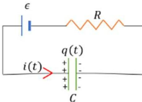
Let the potential across the capacitor be at time  $t$  be  $V_c$ . Let the charge at time  $t$  be  $q$ . The initial charge is  $Q$ .
