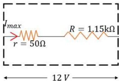
The maximum potential difference that can be measured is  $V_{max} = 12V$ , and let the current through the voltmeter for maximum deflection be  $I_{max}$ .
