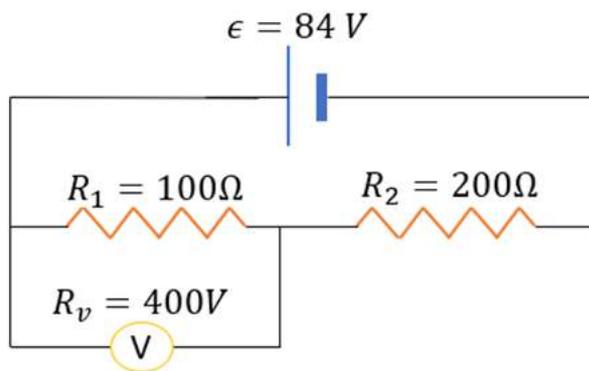
We can easily see that the voltmeter and  $R_1$  are in parallel. The equivalent resistance,  $r'$  is given by:
