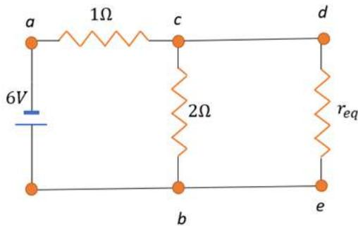
Note that  $de$  and  $cb$  are in parallel. The equivalent resistance is given by:
