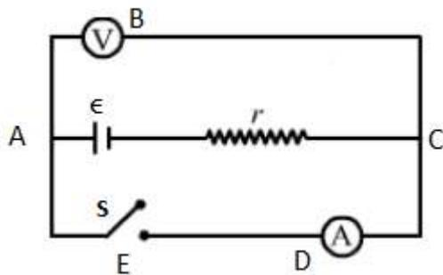
a) When switch is open, the current would circulate through loop ABCA but not through the loop ACDEA. Since the internal resistance is very small compared to the resistance of Voltmeter, the voltage drop occurs completely across the voltmeter. This voltage drop will be measured in the meter and it will be almost equal to the emf of the cell.
