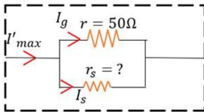
The maximum current that can be measured is  $I'_{max} = 2A$ .
