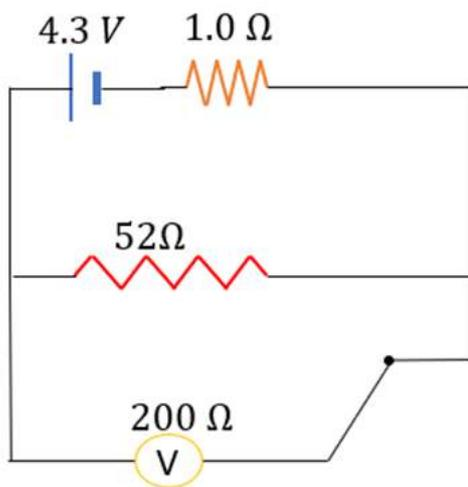
Note that the voltmeter and  $r'$  are in parallel.
