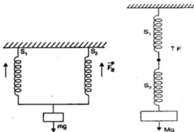
Consider the body of mass  $M$  suspended by two springs connected in parallel. Let  $K_1$  and  $K_2$  be the spring constants of two springs.
