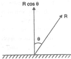
Let  $R$  represents the reaction offered by the ground. The vertical component  $R \cos \theta$  will balance the weight of the person and the horizontal component  $R \sin \theta$  will help the person to walk forward.
