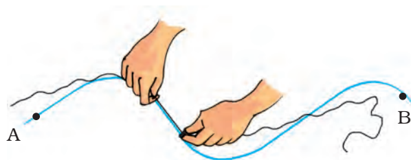
Fig.10.10 Measuring the length of a curved line with a thread
