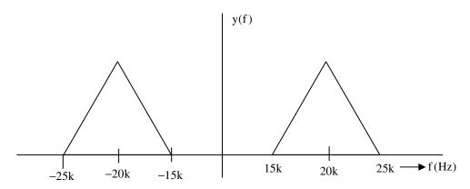
If y(t) is sampled with a sampling frequency ' $f_s$ ' then the resultant signal is a periodic extension of successive replica of y(f) with a period ' $f_s$ '.
