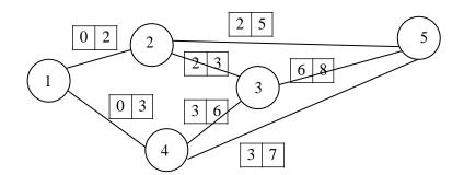
Critical path-1-4-3-5 Time taken = 8 days 51. For flow through a pipe of radius R, the velocity and temperature distribution are as follows:
