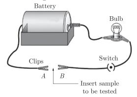
When ...... wire is placed between the terminals A and B. The bulb light up.
