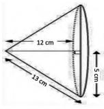
radius r = 5 cm height h = 12 cm and slant height l = 13cm Now, volume of the cone =  $\pi r^2 h/3$
