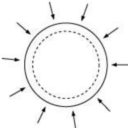
$$B = \frac{\text{Normal stress}}{\text{Volumetric strain}} = \frac{\Delta P}{-\frac{\Delta V}{V}} = -V \frac{\Delta P}{\Delta V}$$
