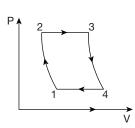
$$\begin{aligned} \frac{cp}{cv} &= 1.4 \\ T_1 &= 300 \text{ YK} \\ T_2 &= 1500 \text{ YK} \\ T_2 &= ? \ T_4 &= ? \\ \frac{T_2}{T_1} &= \left(\frac{P_2}{P_1}\right)^{\frac{Y-1}{Y}} = \left(\frac{6}{1}\right)^{\frac{0.4}{1.4}} = 1.6685 \\ T_2 &= 1.6685 \times 300 = 500.5 \text{K} \\ \frac{T_3}{T_4} &= \left(\frac{P_3}{P_1}\right)^{\frac{Y-1}{Y}} = \left(\frac{6}{1}\right)^{\frac{Y-1}{Y}} = 1.665 \\ T_4 &= \frac{1500}{1.66} = 903.61 \text{ K} \end{aligned}$$
