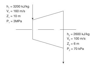
32. If mass flow rate of steam through the turbine is 15 kg/s, the power output of the turbine is (in MW) (A) 9.1 (B) 10.5
