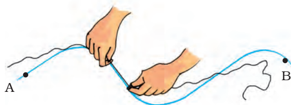
Fig.10.10 Measuring the length of a curved line with a thread
