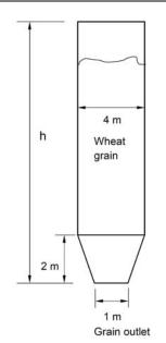
A circular grain silo with conical bottom, as shown in figure, is filled with wheat (true density  $1200 \text{ kg m}^{-3}$ ) with porosity of 0.6. Five hundred metric tonne of wheat fills 80% of its capacity (by volume). The total height (h) of the silo from its grain outlet end in m is \_\_\_\_\_\_.
